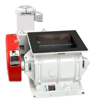
Outboard press fit bearings provide better protection, resulting in longer service life. Special wear resistant MD designs are designed to be placed in abrasive environments. Field tests of these designs show a lifespan up to eight times longer than a standard MD airlock.
