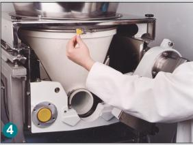
Release band clamp lever for hopper removal.
