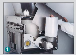
All components are accessible from the rear of the feeder instead of the discharge side. Simply remove back panel and loosen bolt.
