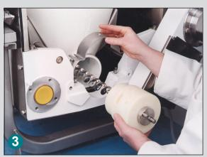
Helix is easily removed allowing for quick helix style and diameter changes.
