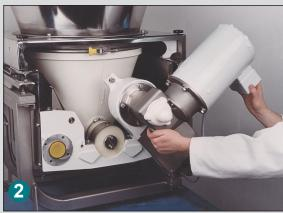
Motor and drive assembly swings back for complete access to all internal components for cleaning, reconfiguration or maintenance.
