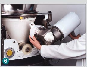
Reposition motor and drive assembly. Tighten bolt and you're ready to run – all in under two minutes.
