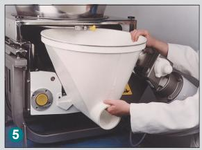
Hopper slides out for easy cleaning, replacement or maintenance.
