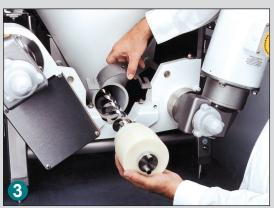
Helix is easily removed allowing for fast and easy helix cleaning and changeover.
