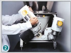
Motor and drive assembly swings to the side for complete access to all internal components for easy cleaning, reconfiguration or maintenance.
