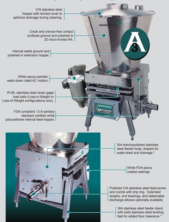
NOTE: Electropolishing, passivation, and other surface preparations are optionally available. \* 316 or 316L stainless steel is optionally available.
