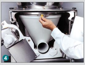
Release band clamp lever for hopper removal.
