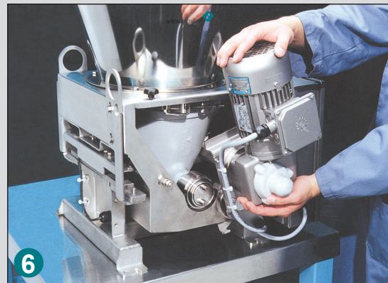
6 Replace components, reposition motor and drive assembly, tighten quill nut, replace backplate and you're ready to run – all in under two minutes.
